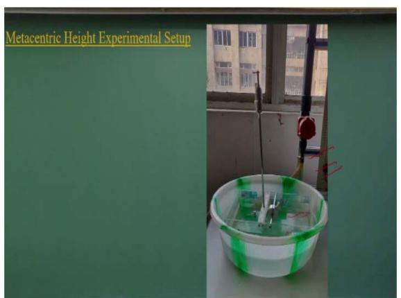
So let us look at simple experiment, metacentric height experimental setups with just balancing the weight we can measure the metacentric height of a floating object like this and this type of facilities are there any fluid mechanics lab, you can just measure the metacentric height and find out the stability of floating object.
