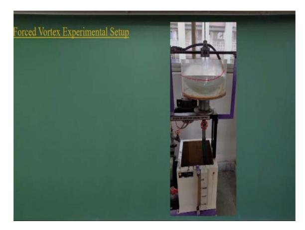
Or you can see this type of forced vortex experimental setups which will be having a motor arrangement to make a uniform rotation. Then to measure the shape of the free surface with a gauging systems. With different rotations you can have a different free surface and you can compare with the theoretical value whether what you are getting from experimental do they match each other.
