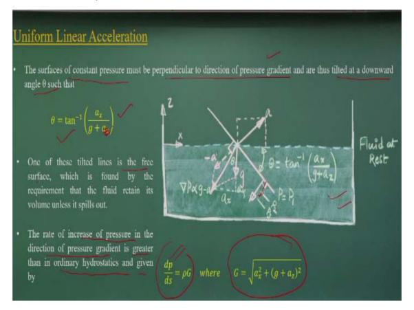
And that is what is the explanations that the surface of the constant pressure must be perpendicular to the pressure of gravity and it will be tilted downward such a way that theta is this part x a z okay, it will be z here. So  $\tan \theta$  will be same diagrams. So if you
