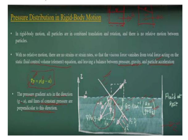
Now let us come it to the another component on fluid statics that means fluid at the rest. But we are looking it a rigid body motions. That means what it happens that if I have a half filled liquid containers. That means I have a half filled liquid containers. It has a free surface and this is the containers. If I accelerate it with acceleration a. Okay, I have a tank and I am just accelerating with acceleration a.
