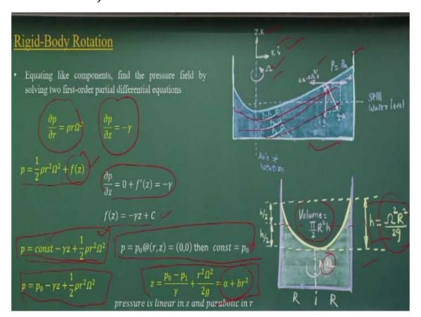
Now let us show it the solving this part. We can solve this one pressure field considering two equations, component wise. Okay one is a z component another is i r component.
